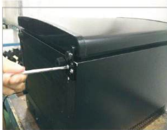
7. Secure the bottom hinge with 3 screws
